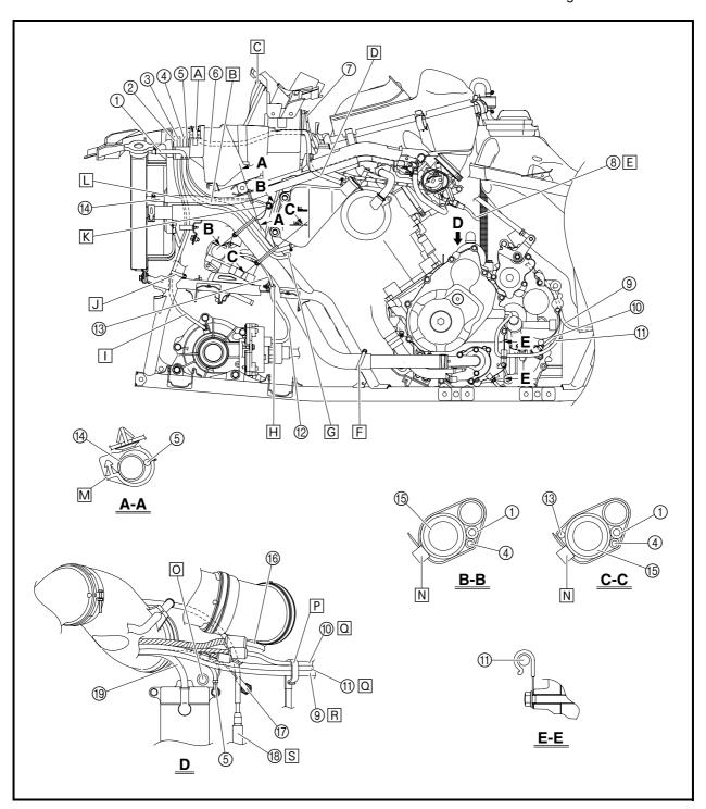
S Route the shift control cable under the gear position switch lead, speed sensor lead, and crankshaft position sensor lead.
