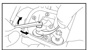
c. Measure the valve clearance with a thickness gauge ①.
