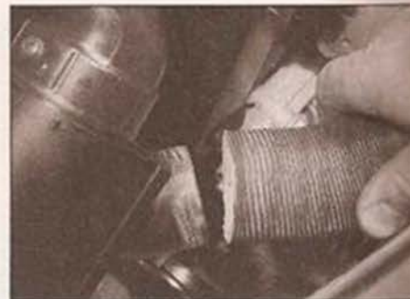
2.9c Pulling off the warm-air duct from the temperature control valve housing
