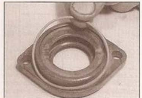
7.3d . . . then recover the O-ring seal
