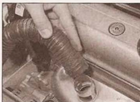
2.8b The warm-air duct is simply pulled off the collector plate stub
