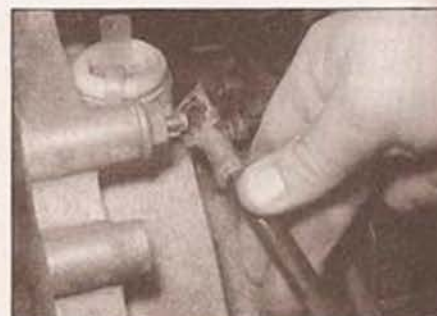
2.29b . . . and disconnect the transmission earth strap
