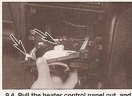
9.4 Pull the heater control panel out, and disconnect the wiring plugs for the heater fan and panel illumination (arrowed)
