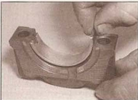
11.8 Fit the new lower half main bearing shells to the main bearing caps
