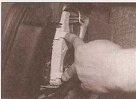
7.27 ... press the bulbholder lugs as shown ...
