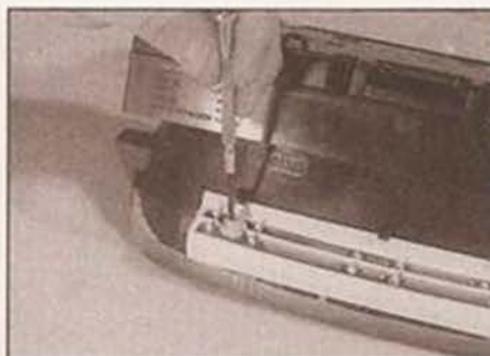
8.11a Turn the bulbholder using a small screwdriver ...
