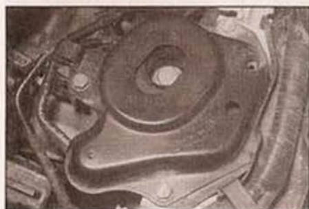
13.13a Two of the transmission left-hand mounting bolts are hidden under the wiring harness plastic guide ...
