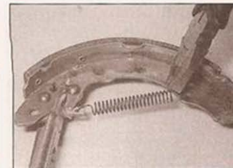
5.18 Fit the spring to the wedge key, and hook it onto the trailing shoe
