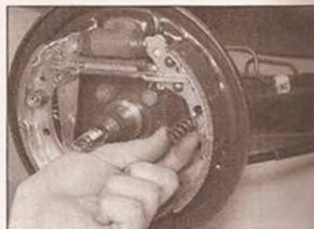
5.7b ... then lift off the spring ...
