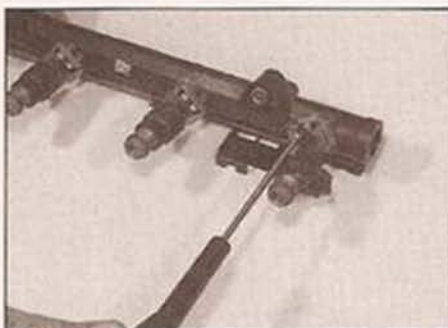
5.15a Using a suitable screwdriver, prise out the injector securing clip ...
