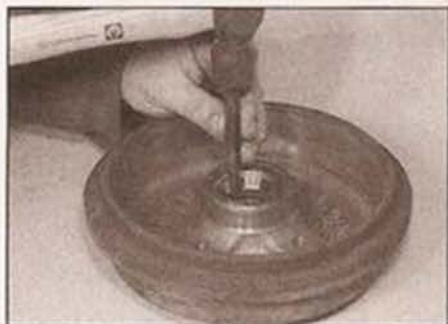
8.3 Drive out the old outer races using a hammer and punch
