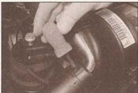
2.9a Removing the screw securing the duct to the air temperature control valve housing
