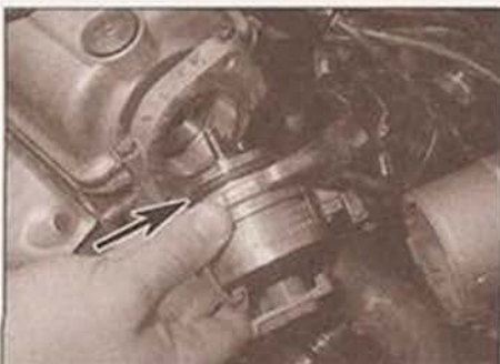
4.8b ... and remove the distributor - note the large O-ring seal (arrowed)
