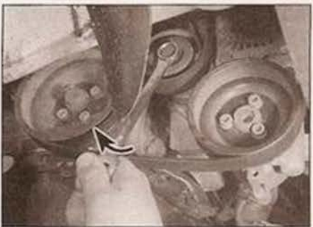
6.8 Rotate the auxiliary drivebelt tensioner clockwise to relieve the tension on the belt
