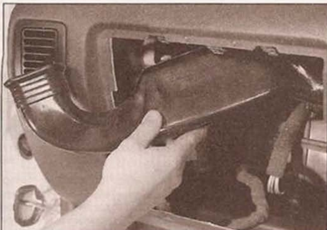
28.17a Removing the vent duct through the glovebox aperture ...
