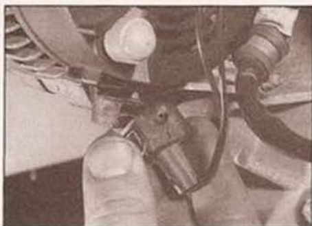
5.3 Unplug the sense cable from the alternator at the connector (later diesel engine model shown)
