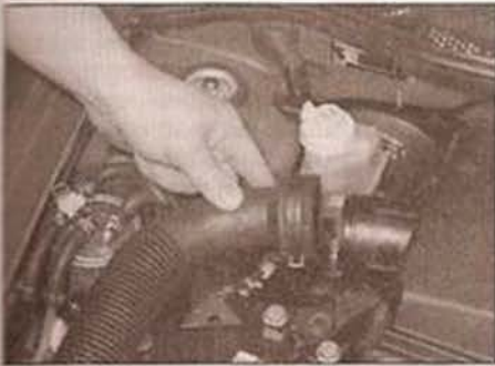
11.6 Disconnecting the inlet air trunking from the inlet manifold cover
