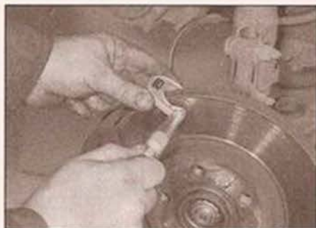
6.3 Measuring brake disc thickness with a micrometer
