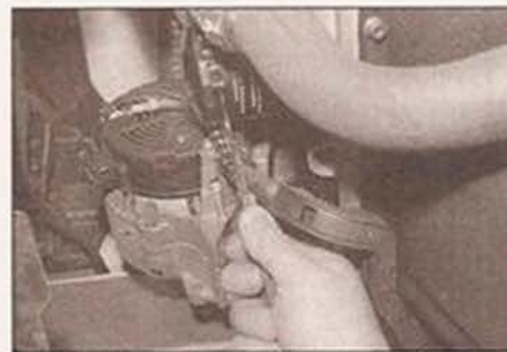
3.8 Loosening the oil filter using a chain-type removal tool
