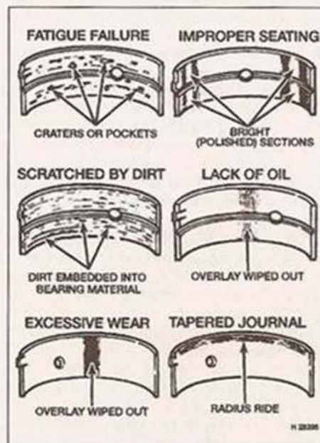
9.1 Typical bearing failures
