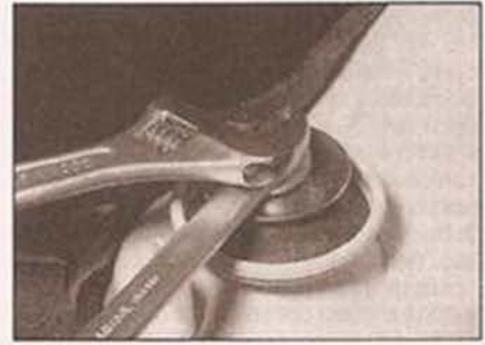
10.6 Hold the piston rod stationary using a suitable spanner, and unscrew the upper mounting nut
