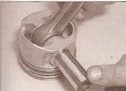
5.12b Push out the gudgeon pin and separate the piston and connecting rod
