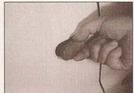
7.20 Push the side repeater light to the rear, and pull out at the front
