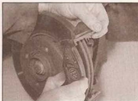
4.11b ... then the upper anti-rattle spring and the outer pad ...
