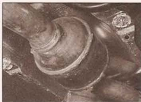
6.1 Oxidation catalyst fitted to diesel engine models
