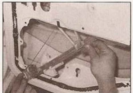
14.23 Removing the rear door window regulator
