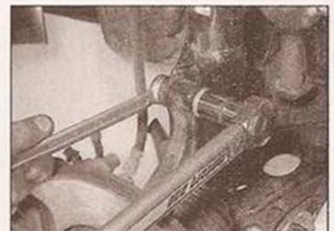
2.7 Tighten the strut-to-swivel hub nuts/bolts to the specified torque
