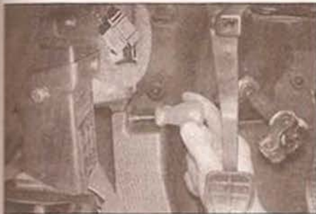
9.29 Removing the screw securing the clutch footrest to the air distribution housing
