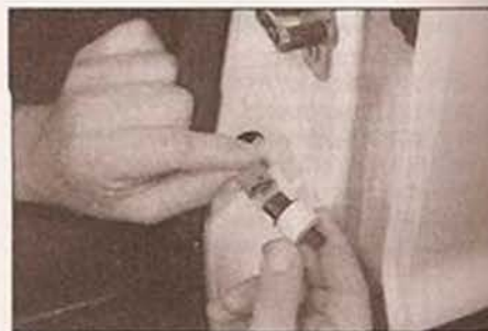
6.11 Disconnect the switch wiring, but make sure it does not fall back into the pillar
