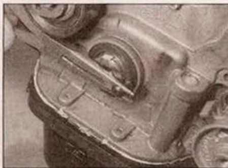
9.5b ... and pull out the seal using pliers
