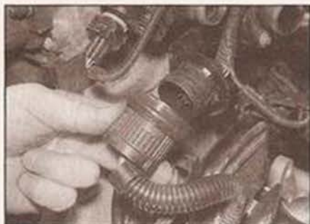
2.20 Unscrew the bayonet-fit main wiring harness connector from the left-hand end of the cylinder head
