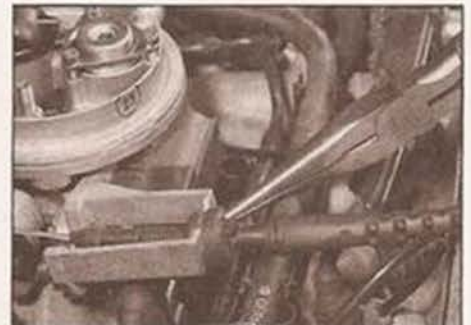
4.9 Adjust the accelerator cable by inserting the metal clip into one of the slots in the cable outer
