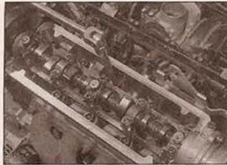
10.20b Loosen the bolts by half a turn at a time, using a suitable splined adapter
