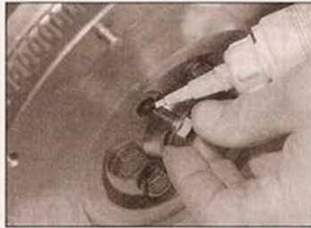
12.7 Apply locking fluid to the new flywheel bolts, if necessary
