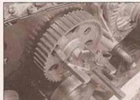
6.8 Attach a two-legged puller to the injection pump sprocket
