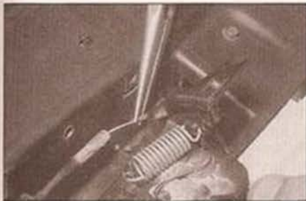
9.1a Unhook the bonnet release inner cable ...
