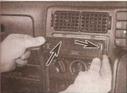
17.4a Withdrawing the radio/cassette from the fascia - removal tool slots arrowed
