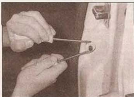
6.10 ... then use two screwdrivers to release the switch from the door pillar
