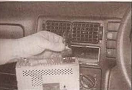
17.4c ... and the supply and speaker connector plug, and remove the unit from the fascia
