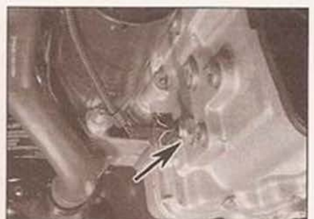
14.3 Reversing light switch (arrowed) - seen from below
