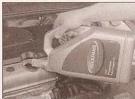
3.12b ... then fill the engine using the correct grade and quantity of oil
