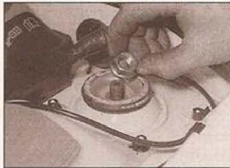
2.3b . . . loosen and remove the strut upper mounting nut
