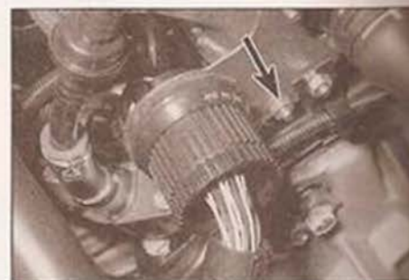
6.15b Main harness wiring connector at left-hand end of cylinder head, and earth connection (arrowed)
