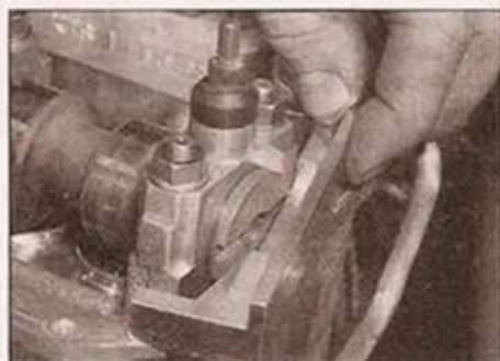
2.4 Engage the locking bar with the slot in the camshaft
