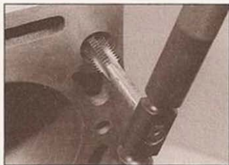
8.6 To clean the cylinder block threads, run a correct-size tap into the holes
