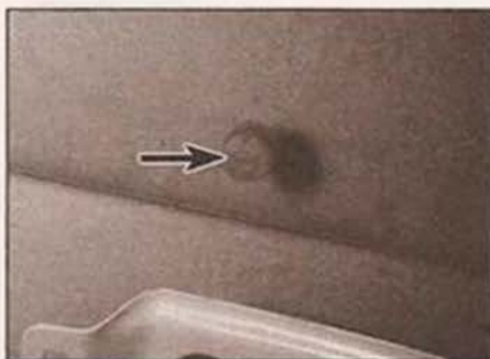
14.29 Fit the plastic plug and spreader pin (arrowed) so that they protrude an equal amount either side of the glass
