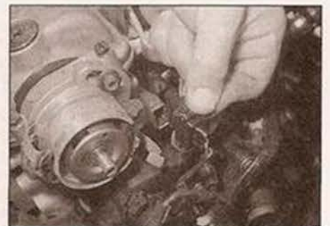
10.8e . . . distributor Hall sensor wiring plug . . .
