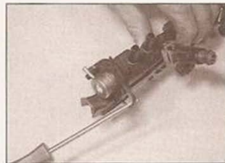
5.23b To remove the pressure regulator, prise out the retaining clip and withdraw it from the fuel rail
