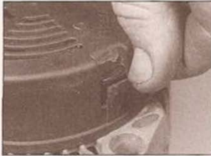
6.3b . . . then prise open the clips . . .
