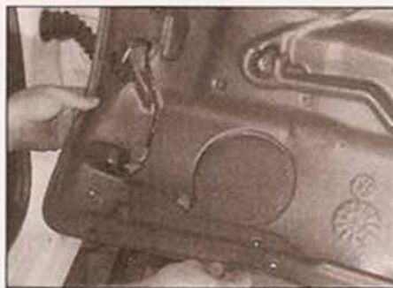
14.4b Removing the foam panel
