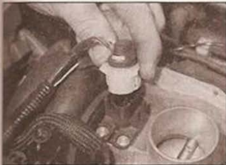
5.4a Disconnect the throttle potentiometer wiring plug . . .
