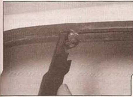
14.14 Pull the guide channel downwards...
