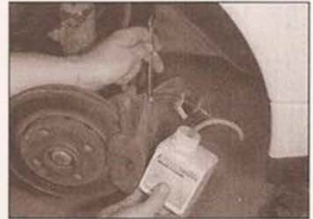
2.22 Bleeding front brake caliper using a one-way valve brake bleeder kit
