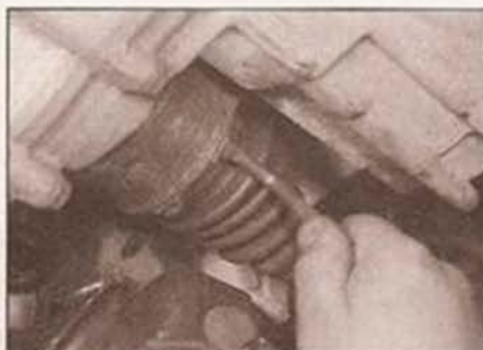
2.7b Using a suitable key or socket, slacken the splined bolts...
