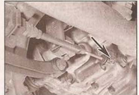
3.15 Prise off the retaining circlip and lever off the transmission support cable - renew bush in cable end fitting (arrowed)
