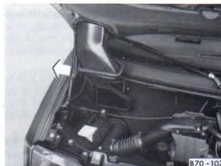
**To close** bonnet lift it slightly and pull the strut forward – see illustration. Let bonnet drop into locks from a height of about 30 cm – do not press it closed.
