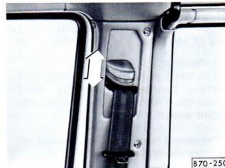
With the aid of the **belt height adjustment** the routing of the front seat shoulder belt can be set to fit the body properly.
