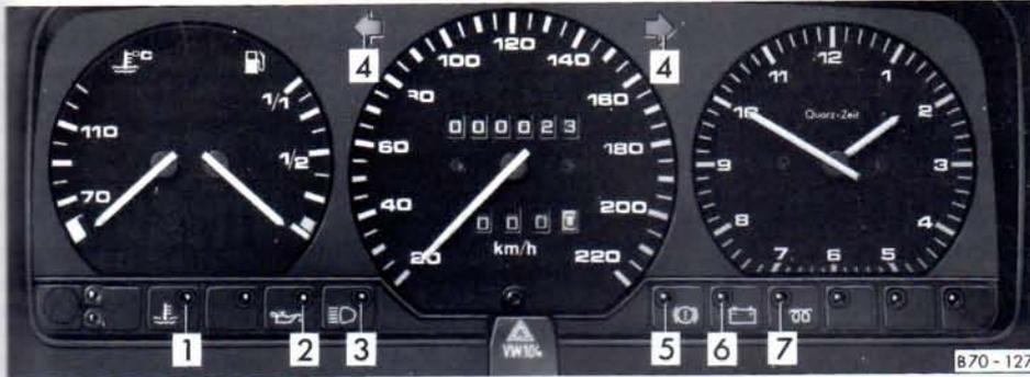
The layout of the warning lamps depends on the model and the engine fitted. The symbols shown here are also on the actual warning lamps.
