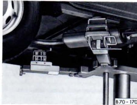
Short wheelbase vehicles, when unladen can as an exception be lifted on a single column hoist.
