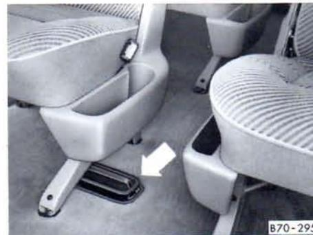
On vehicles with seating arrangement the outlet is located under the centre row of seats. This outlet can be closed by pushing it in.
