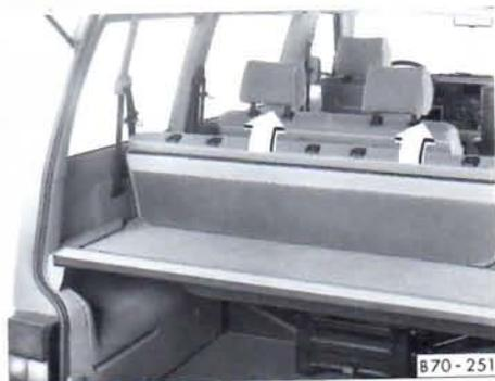
The rear seat backrest with a loading/sleeping surface can be folded forward to provide a large loading and/or sleeping surface.
