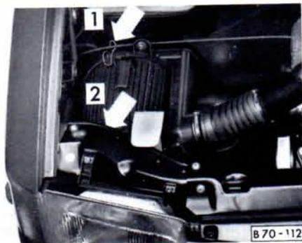
The paper filter element in the air cleaner is normally renewed as detailed in the Service Schedule. In very dusty conditions the element must be cleaned or renewed at shorter intervals.
