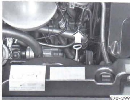
The engine must be running at idling speed, the handbrake must be applied and the selector lever at "N".
