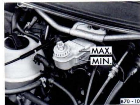
The brake fluid reservoir is in the engine compartment.
