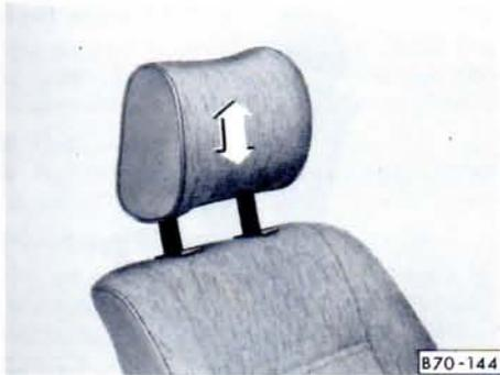
The front head restraints are adjustable for rake and height and should be set to suit the size of the person in the seat. Correctly adjusted head restraints together with the seat belts offer effective protection.
