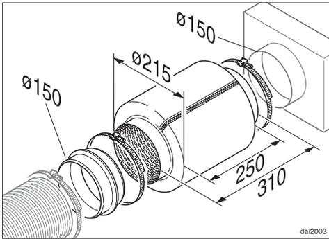
To reduce noise levels even further, a silencer (optional accessory) can be installed in the exhaust ducting.
