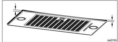
If the installation surface is uneven making flush installation difficult, the frame can be realigned.
