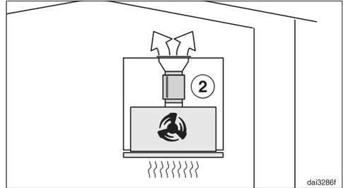
In recirculation mode, the silencer needs to be positioned between the exhaust vent and the exhaust grille ②. Check that there is sufficient space.
