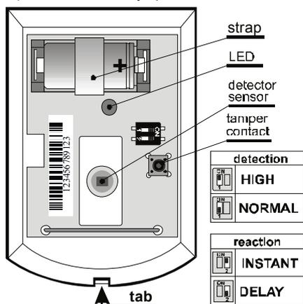
To observe EN 50131-2-2 the battery in the JA-83P must be fixed with the supplied strap and the tabs must be secured by the supplied screw.
